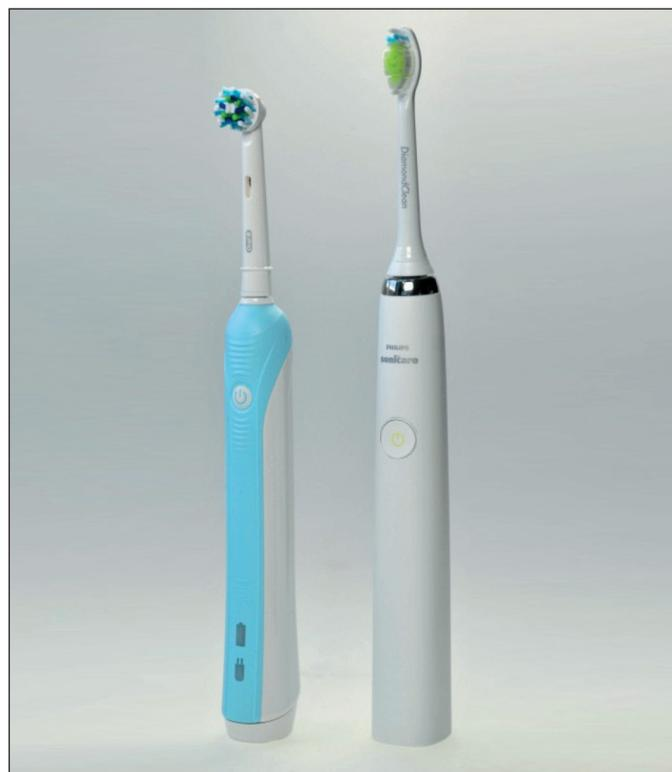
**Figure 1.** Oscillating-rotating (left) and sonic (right) test toothbrushes.
